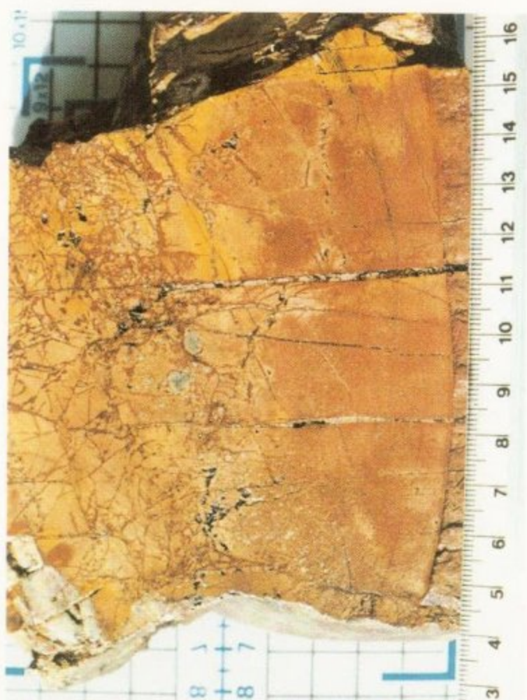
A. Quartz-pyrite-cassiterite vein and intensive wall-rock alteration in Mount Wells Tin Mine (see Figure 2). B. Gold-bearing quartz vein cutting hydrothermal alteration in the hinge of anticline. Spring Hill Gold Mine – main shaft (see Figure 2). C. Folded and dislocated quartz veins within the bedding of Koolpin Formation. Spring Hill Gold Mine – old tin workings 700 m from the main shaft (see Figure 2). D. Stockwork of quartz veinlets cutting sediments of the Koolpin Formation. Spring Hill Gold Mine – old tin workings 700 m from the main shaft (see Figure 2).
