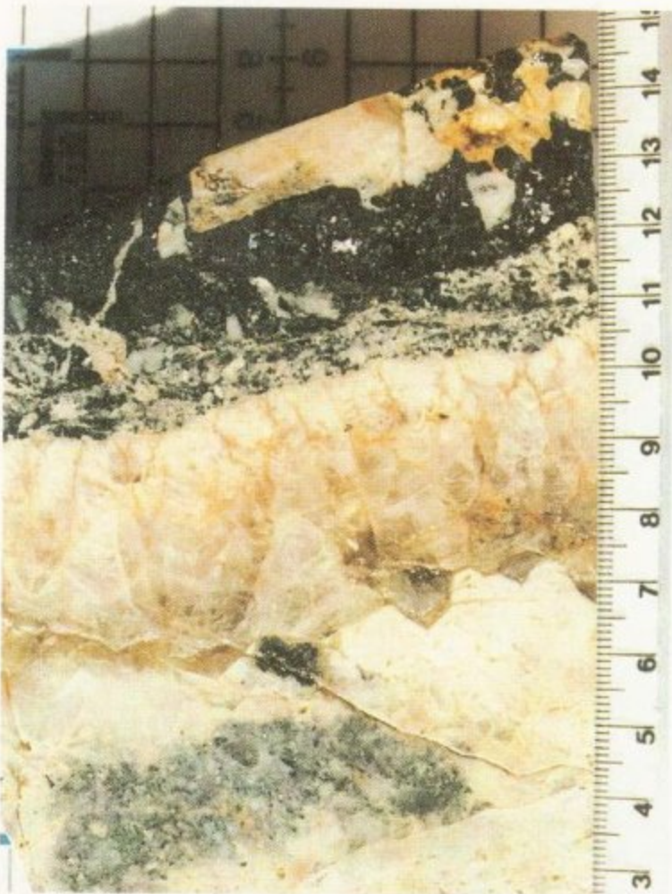
A. Quartz perimorphs after calcite (barite ?). Epithermal quartz vein in the Lead Prospect, Mount Shoobridge area (see Figure 13). B. Zonal crystals of smoky quartz in the margin of the epithermal quartz vein. Lead Prospect – Mount Shoobridge area. C. Quartz crystals and galena in epithermal quartz vein from Lead Prospect – Mount Shoobridge area. D. Perimorphs of quartz after calcite (barite ?) in epithermal quartz vein in the Lead Prospect (Mount Shoobridge area).
