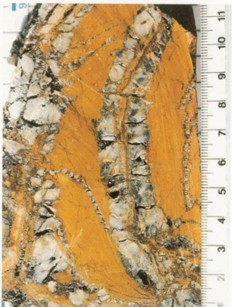
A. Quartz-pyrite-cassiterite vein and intensive wall-rock alteration in Mount Wells Tin Mine (see Figure 2). B. Gold-bearing quartz vein cutting hydrothermal alteration in the hinge of anticline. Spring Hill Gold Mine – main shaft (see Figure 2). C. Folded and dislocated quartz veins within the bedding of Koolpin Formation. Spring Hill Gold Mine – old tin workings 700 m from the main shaft (see Figure 2). D. Stockwork of quartz veinlets cutting sediments of the Koolpin Formation. Spring Hill Gold Mine – old tin workings 700 m from the main shaft (see Figure 2).
