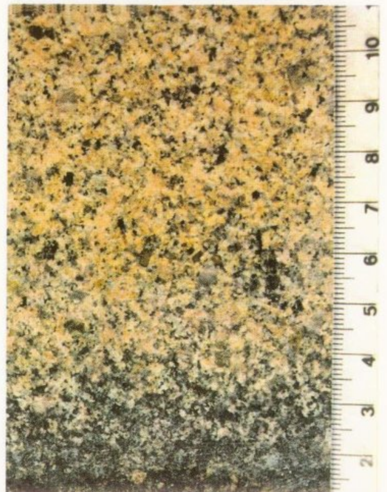
A. Contact between Frances Creek Granite (YIS) and Minglo Granite in the sample locality G-16 (see Appendix III). Biotite rich margin of the younger granite (Frances Creek Granite). B. Biotite granite of the core zone of the Mount Shoobridge pluton intrudes into the marginal biotite-hornblende monzonite. C. Tourmaline breccia with fragments of sandstone from the contact of Allamber Springs Granite (TIS) in sample locality G-26 (see Appendix III). D. Greisenisation of the Yemberrie Granite (YIS) in sample locality G-31 (see Appendix III).
