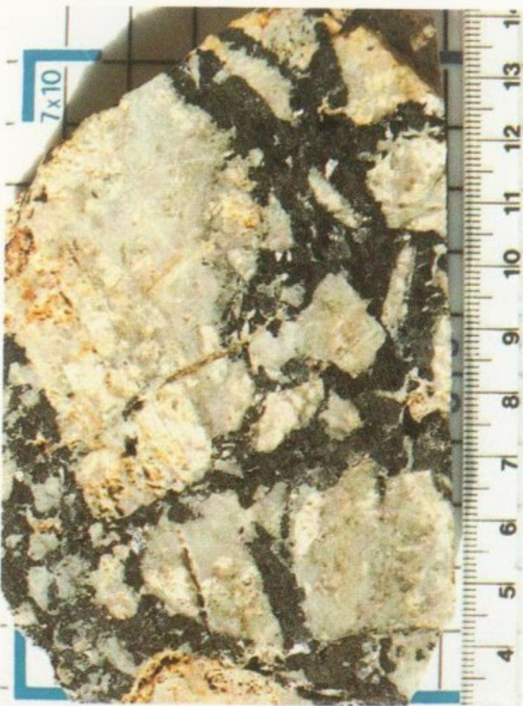
A. Quartz breccia with grains of galena in tourmalinised sediments. Old Company Tin Mine – Mount Shoobridge area (see Figure 13). B. Barite breccia from Copper Prospect - Mount Shoobridge area. C. Granite breccia cemented by galena from epithermal vein in the Burnside Pluton. Lead Prospect – Burnside Pluton (see Figure 11). D. Quartz breccia with galena, sphalerite paramorphism after wurtzite and chalcocite from quartz vein in Rising Tide Prospect – exocontact of the Burnside Pluton (see Figure 11).
