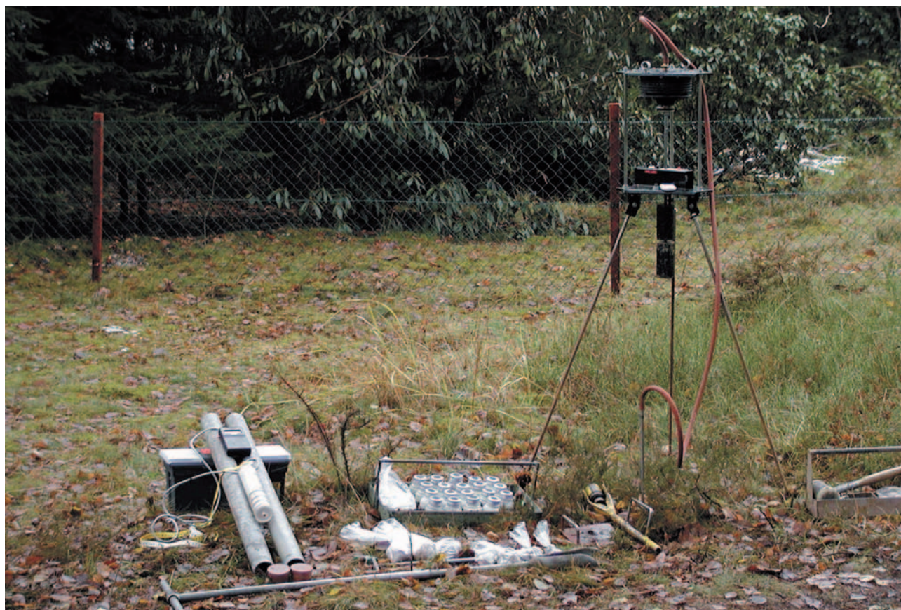
Fig. 5-1. Permeameter RADON JOK and other equipment for in situ measurements.
