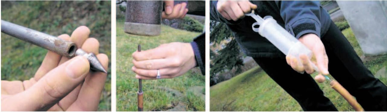
Fig. 3-1. Soil gas sampling: (left) Inserting the sharpened tip into the lower end of the probe. (center) The sharp tip is moved a few centimetres lower – this action creates a cavity at the lower end of the probe. (right) Soil gas sample collection using a syringe.
