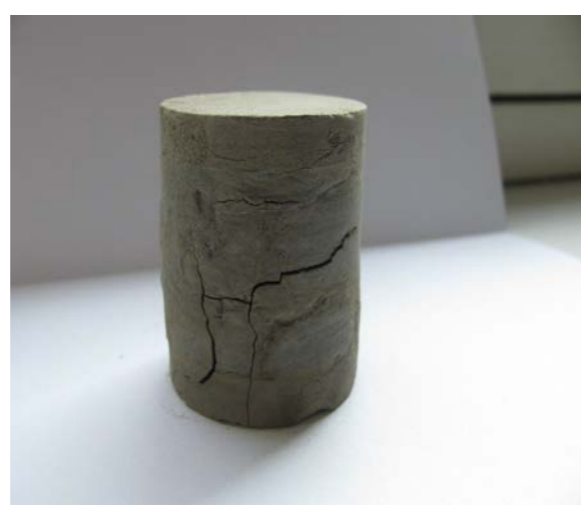
Fig. 3: Photos of sample Hr - 121 before (left) and after (right) long-term dynamic experiments with supercritical CO 2 .
