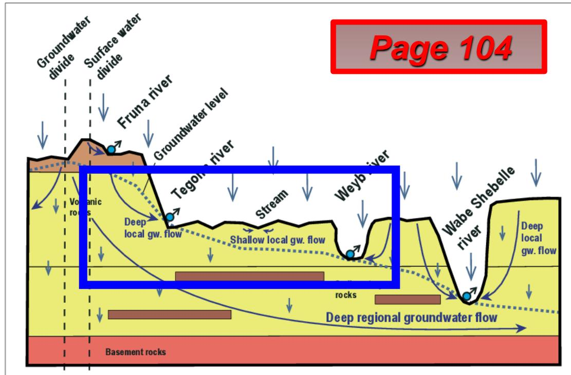
Fig. 4.8 Conceptual hydrogeological model of the Asela highland area
