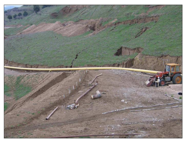
No rotation, only tensile cracks – prevail displacements parallel to slope gradient
