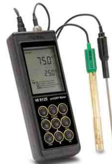
HANNA Multi-meter with fluoride ( F^- ) probe
