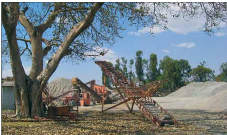
Fig. 4.10 Crushing basaltic rock in the quarry for asphalt and concrete mixes
