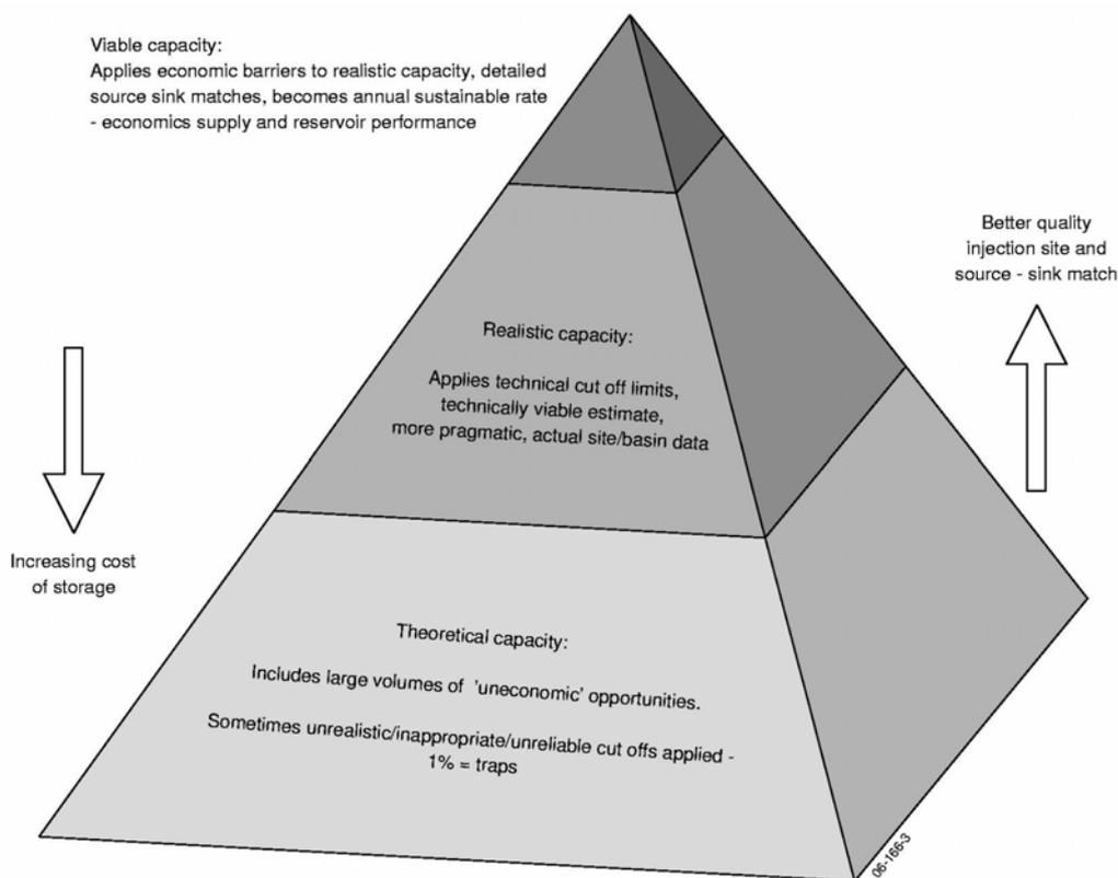
Figure 2 Techno-Economic Resource Pyramid for capacity for CO<sub>2</sub> geological storage, showing the three levels of Theoretical, Realistic and Viable estimates. Theoretical includes the entire pyramid, Realistic the top two portions and Viable only the top portion.
