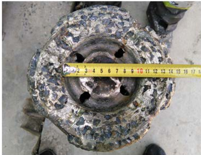
Fig. 5. Wear of the drilling bit during the reopening the well Brodské-72.
