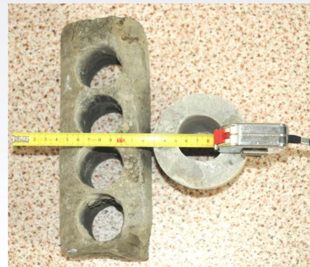
Figure 2. Core residuals after drilling (16 th of June). Similar core drilling residuals are from the other tests as well. This material is to be sent back to Czech Republic.
