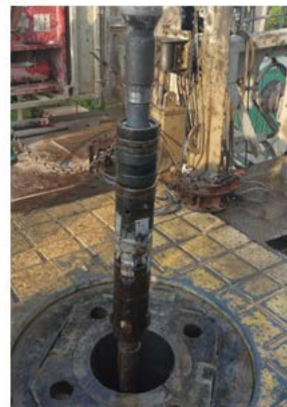
Fig. 8. Launch of the packer in the well Brodské-72.
