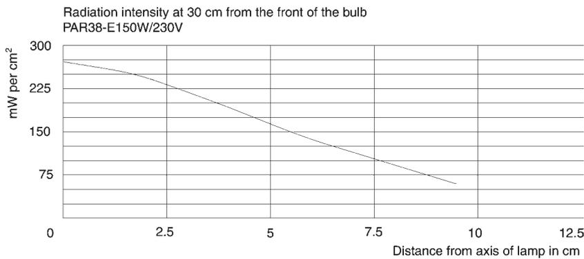
Figure 1. Intensity of infrared radiation: tungsten lamp PAR38-E (Philips).
