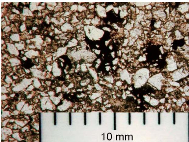
Figure 12. Fine-grained texture of the Maletín Sandstone. Locally formed Fe cement. II N. Photo by P. Pospíšil.
