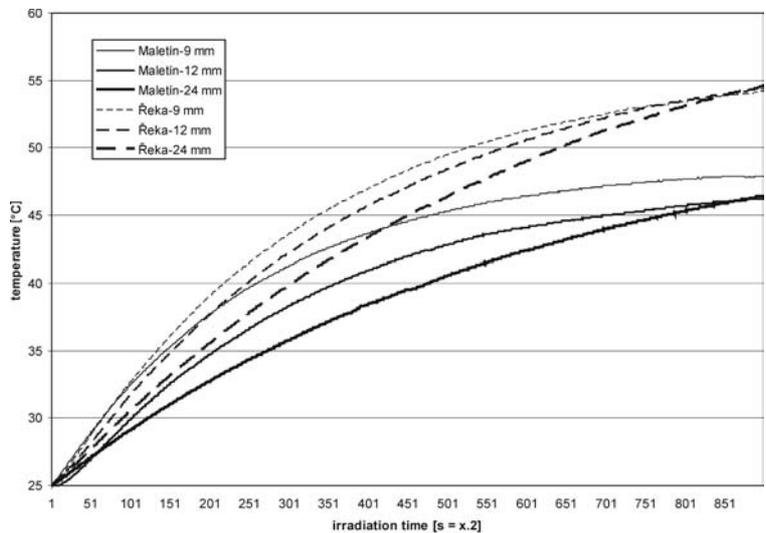
Figure 20. Temperature increase of samples in relation to irradiation time. Dry samples.
