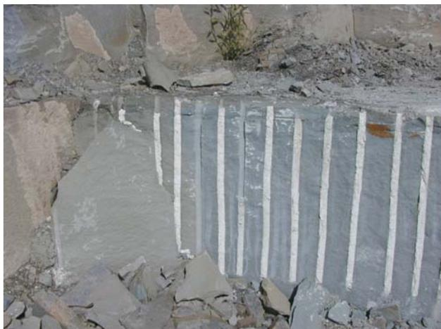
Figure 7. Fresh fracture surface. Godula Sandstone, from the quarry near Řeka. Photo by P. Cikrle.
