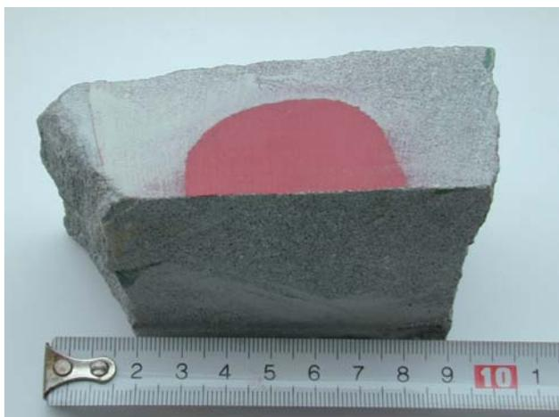
Figure 27. Absorption of nitrocellulose paint by the Godula Sandstone.
