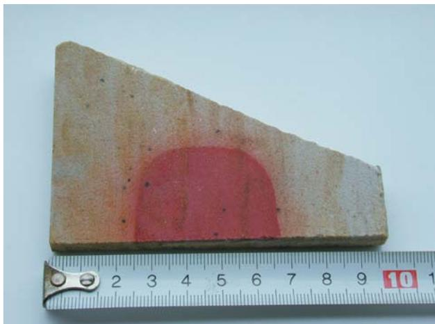
Figure 25. Absorption of nitrocellulose paint by the Maletín Sandstone.
