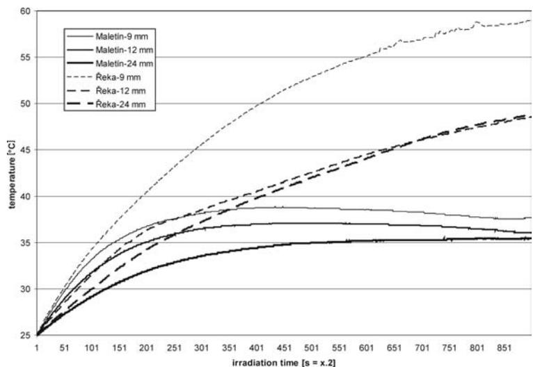
Figure 21. Temperature increase of samples in relation to irradiation time. Water saturated samples.
