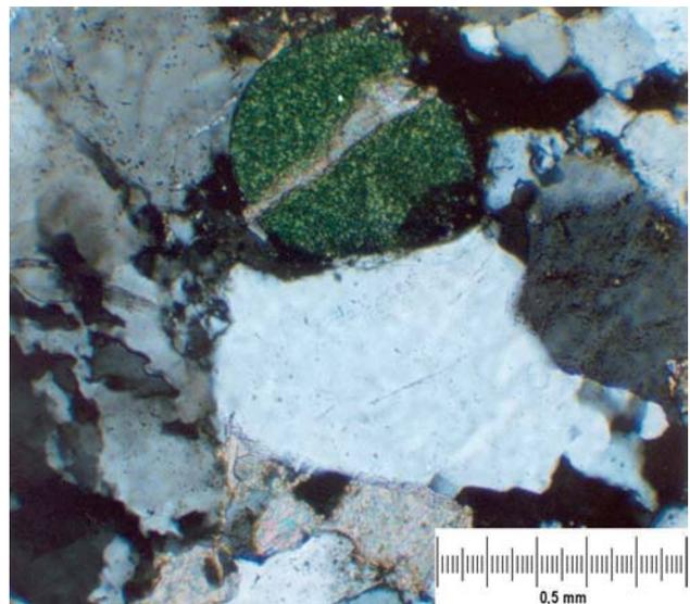
Figure 14. Carbonate cement replacing quartz and rounded glauconite within pores in the medium-grained Godula Sandstone. X N. Photo by P. Pospíšil.
