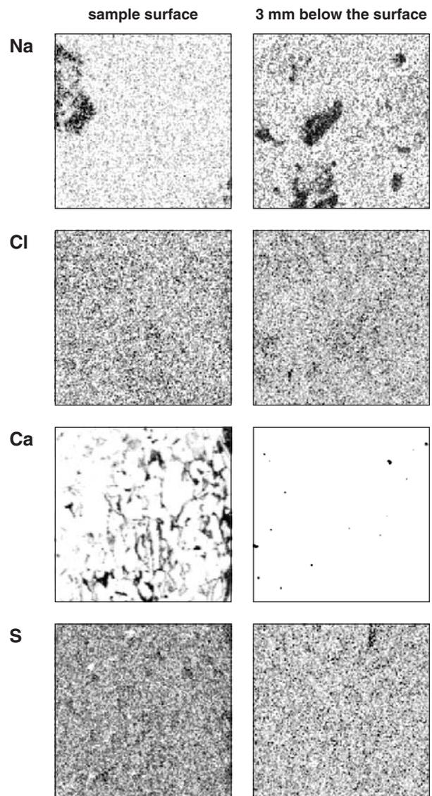
Figure 23. X-ray mapping of sample of weathered Godula Sandstone from the outer cladding of the Military Academy in Brno.
