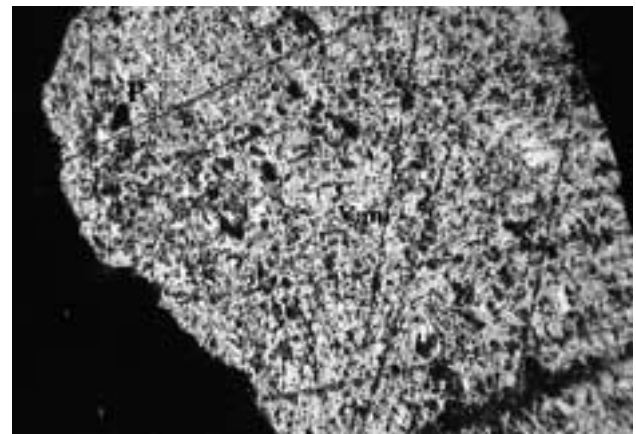
Photo 20. Sample No. 46. Natural high thermal alteration of coal (II/2). Totally thermally metamorphosed coal with character of semi-coke with increasing mean reflectance of metamorphosed vitrinite (Vam) and many fine macropores (P). The texture of coal matter is very homogenous.
