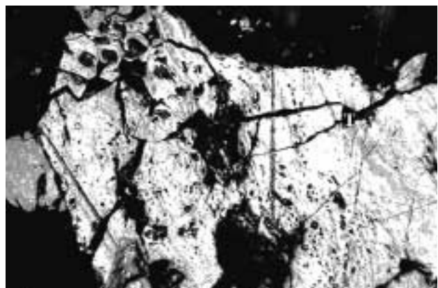
Photo 18. Sample No. 44. Naturally thermally and highly oxidative altered coal (alteration type IV/2). Grains of blanching vitrinite (Va) with contraction cracks (T).
