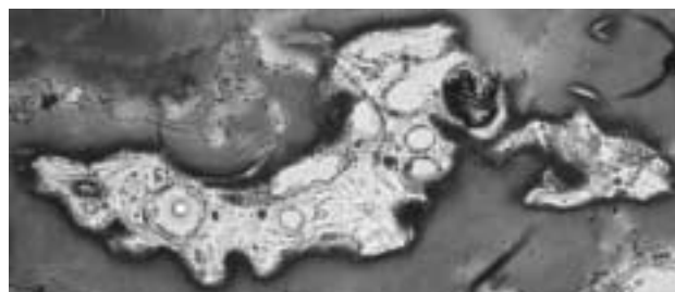
Figure 8. Photomicrograph of fused glass (lechatelierite), Ries, Germany, plane light, field-of-view = 2.5 mm.
