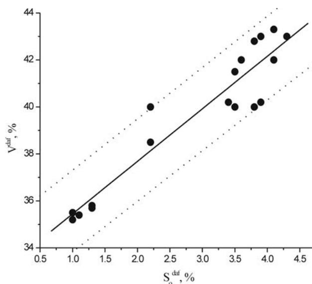
Figure 3. Dependence of the volatile matter yield on the organic sulphur content for G brand coals.
