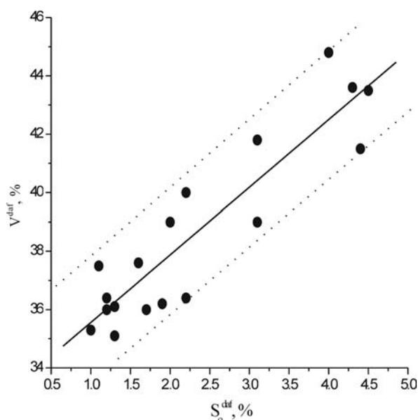
Figure 2. Dependence of the volatile matter yield on the organic sulphur content for DG brand coals.
