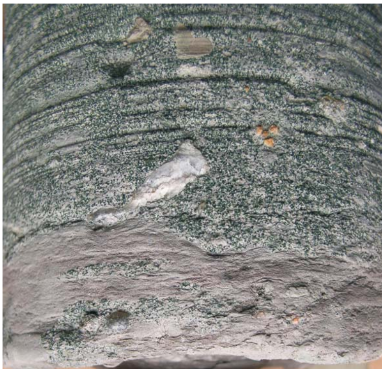
Figure 15. Core photo from borehole Sokoleč OP-3, core interval 63.1–63.25 m. Erosion surface at the base of green glauconitic sandy marlstone (base of Bílá Hora Fm.) with pebbles of quartz and phosphatic nodules. Thalassinoides burrows pipe glauconitic sediment down into the underlying dark grey siltstones of the Pecinov Member. Core is stored at CGS.
